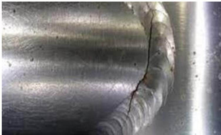
Fig. 3.2.28: Crepa. Fonte: <https://www.rapiddirect.com/blog/types-of-welding-defects/>
