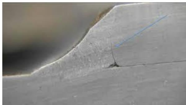
Fig. 3.2.29: Mancanza di fusione. Fonte: <https://www.onestopndt.com/ndt-articles/what-is-lack-of-fusion-in-welds>
